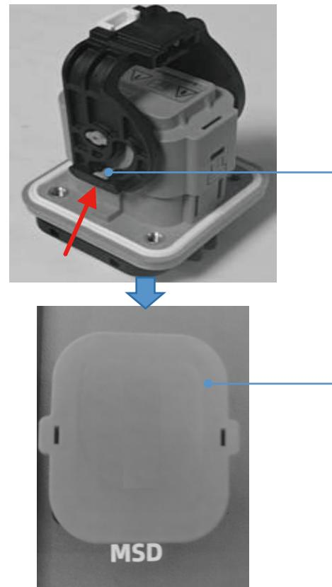
⑤Plug unlocked (Step 4). After separating the plug, collect the MSD plug and store it for protection.
