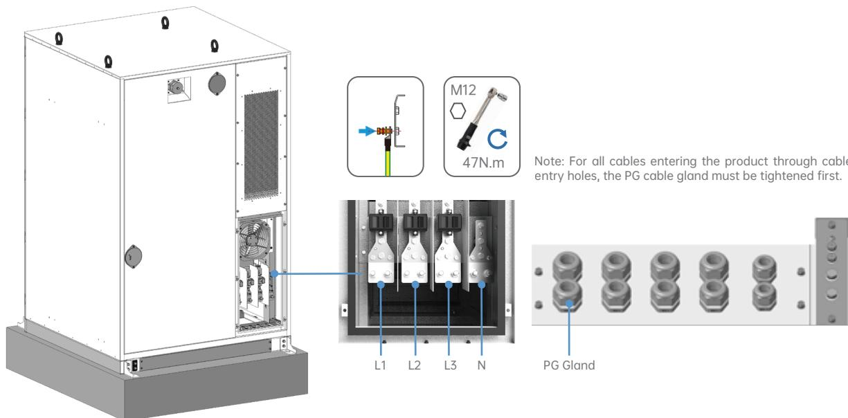
(1)broken. The neutral (N) conductor must be securely connected; otherwise, AC equipment inside the system may be damaged.
