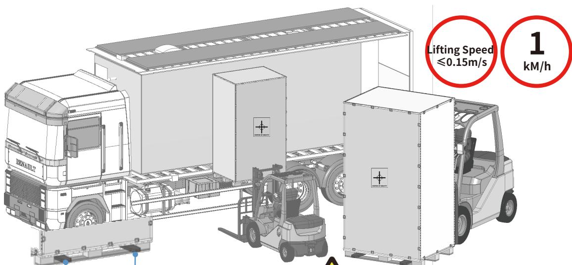
The forklift arms must align closely with both sides of the forklift pockets on the wooden crate or carton base, and the forklift arms must be able to extend fully through the crate.
