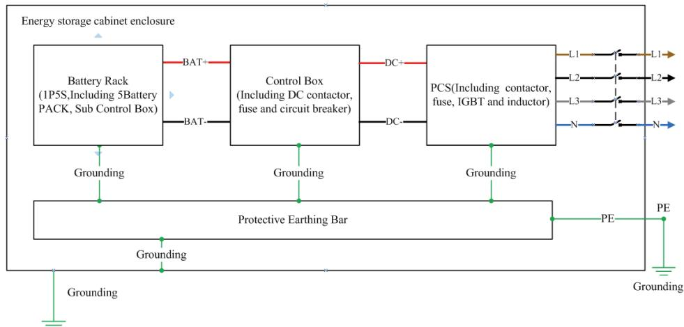
The protective earthing cable shall comply with IEC 60364-5-54:2011/AMD1:2021, IEEE standards, or local regulatory requirements. The grounding resistance between internal equipment and the grounding bar shall be  $<0.1 \Omega$ , and the grounding resistance between the equipment enclosure or ESS grounding bar and the grounding network shall be  $<4 \Omega$ .
