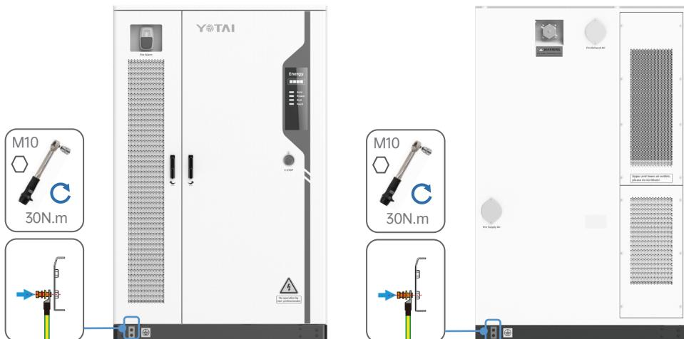
Figure 6-2 Connection of Energy Storage System PE Copper Busbar Protective Earthing Cable
